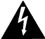
The lightning flash with arrow-head symbol, within an equilateral triangle, is intended to alert the user of the presence of uninsulated "dangerous voltage" within the product's enclosure; that may be of sufficient magnitude to constitute a risk of electric shock to persons.
